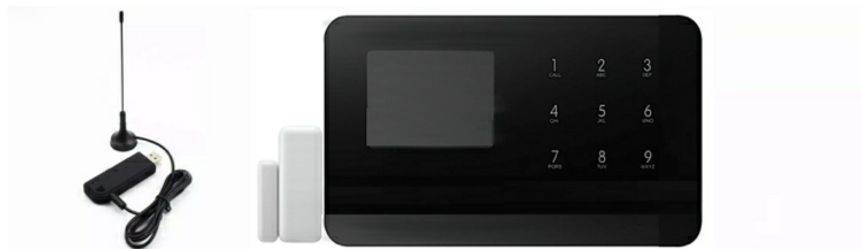
Figure 15-1: A cheap RTL-SDR DVB-T dongle and an alarm system with a wireless door access sensor
