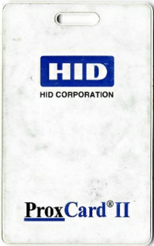
Figure 10-4: The HID ProxCard II, a popular low-frequency RFID tag
