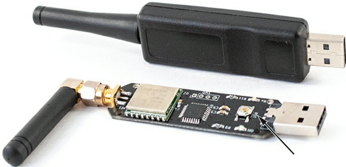
Figure 13-6: The CatWAN USB stick, which is compatible with LoRa and LoRaWAN, is based on the RFM95 transceiver. The arrow points to the reset (RST) button.
