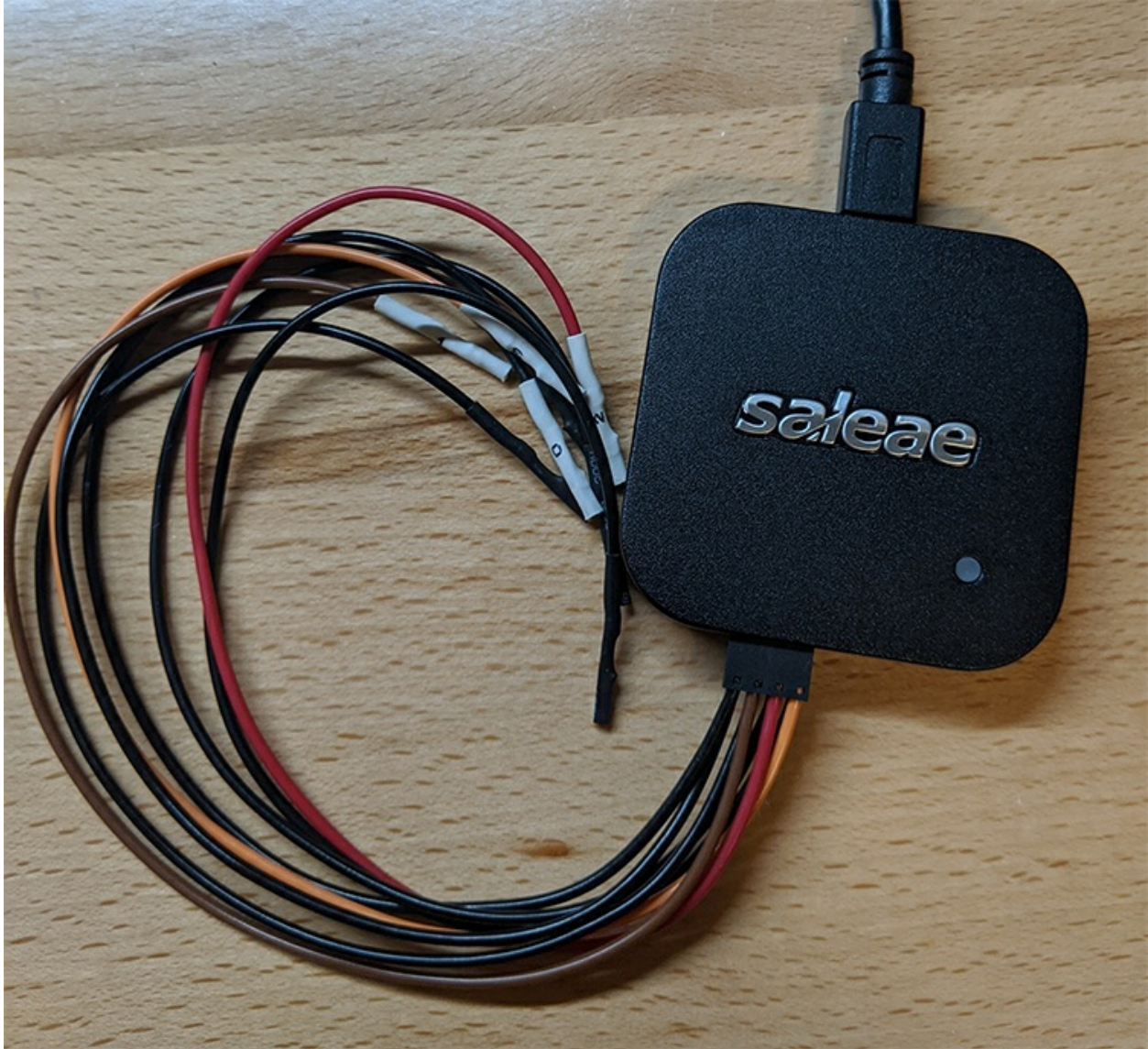
Figure 7-5: Saleae is a family of professional logic analyzers.
