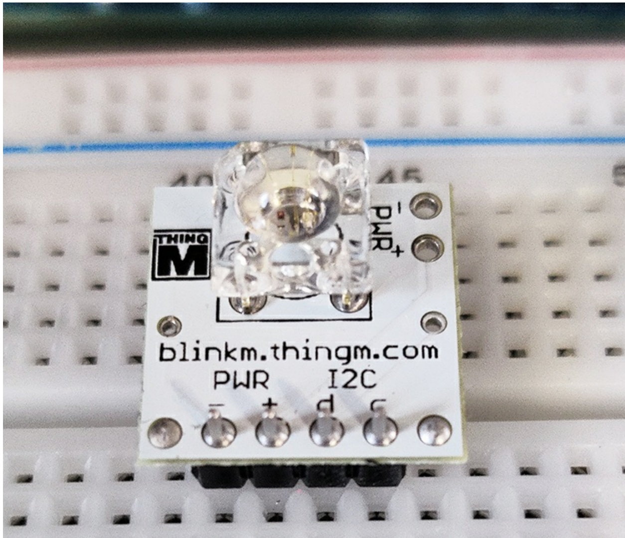
Figure 8-9: We can connect SDA and SCL without resistors because the Arduino pins include built-in resistors.
