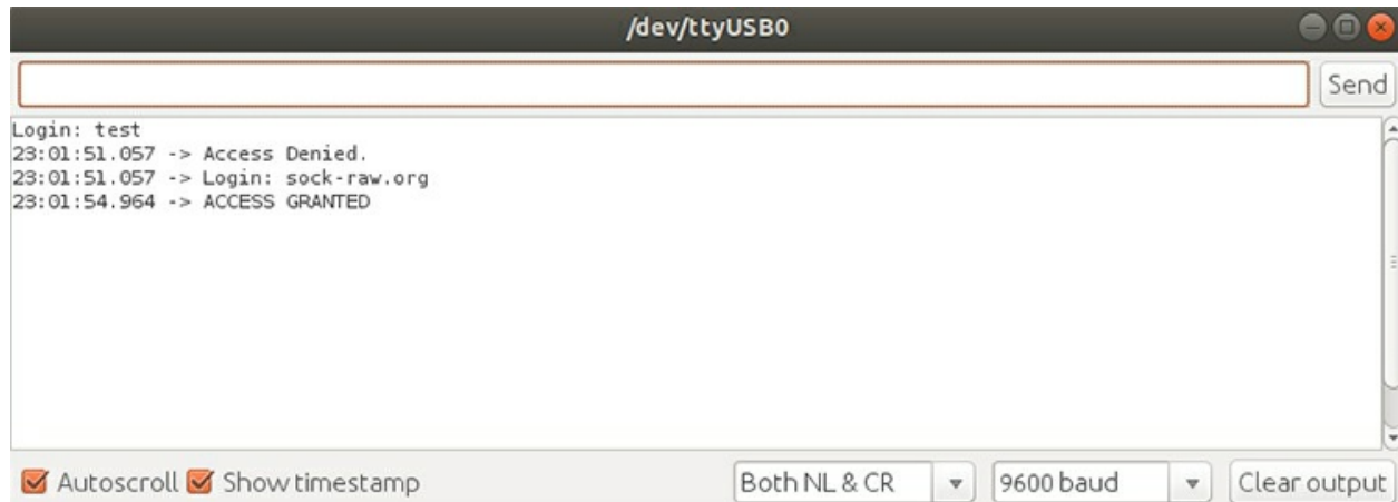
Figure 7-17: The Serial Monitor pop-up window in the Arduino IDE
