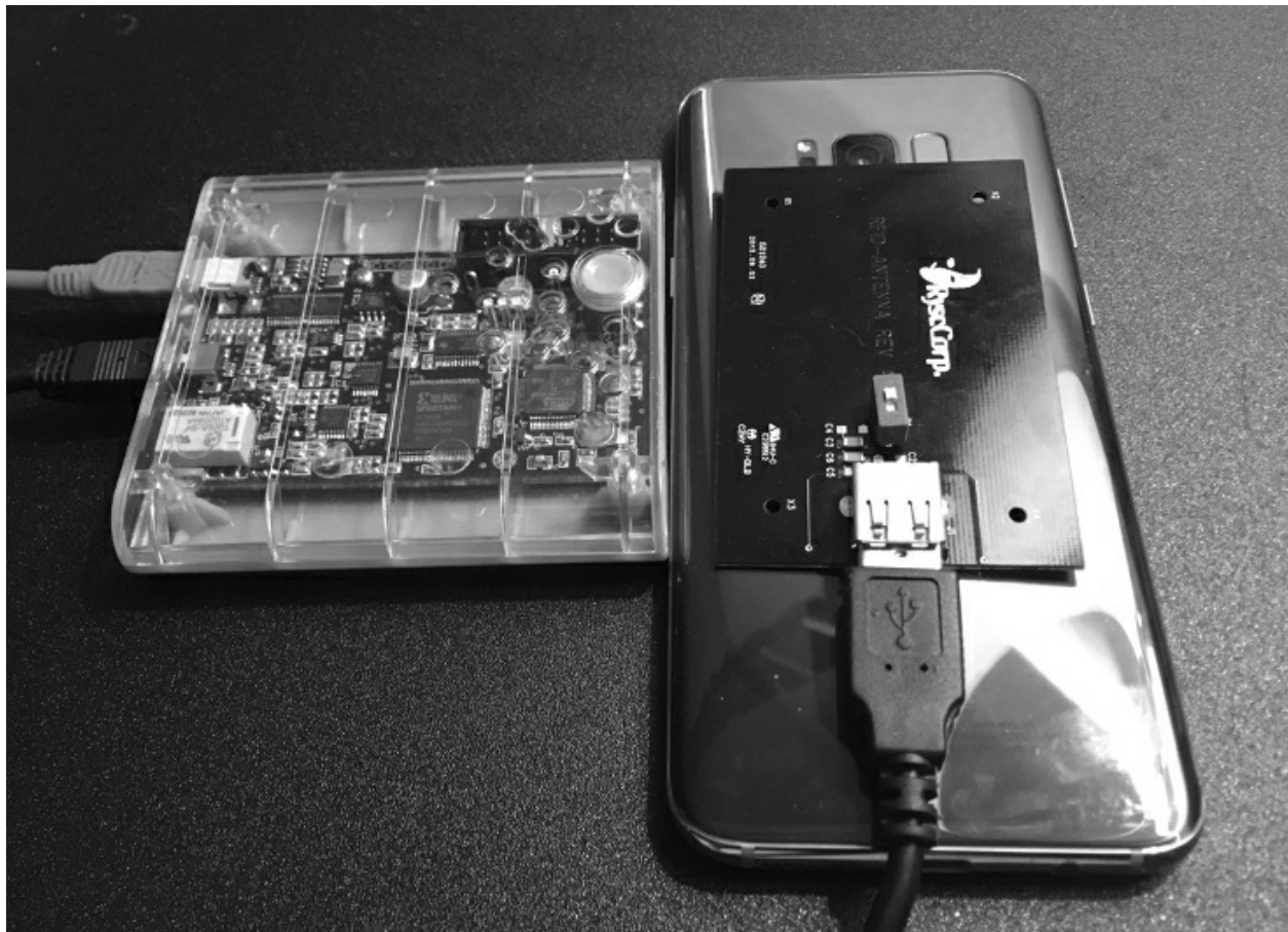
Figure 10-9: Fuzzing the RFID reader in an Android device
