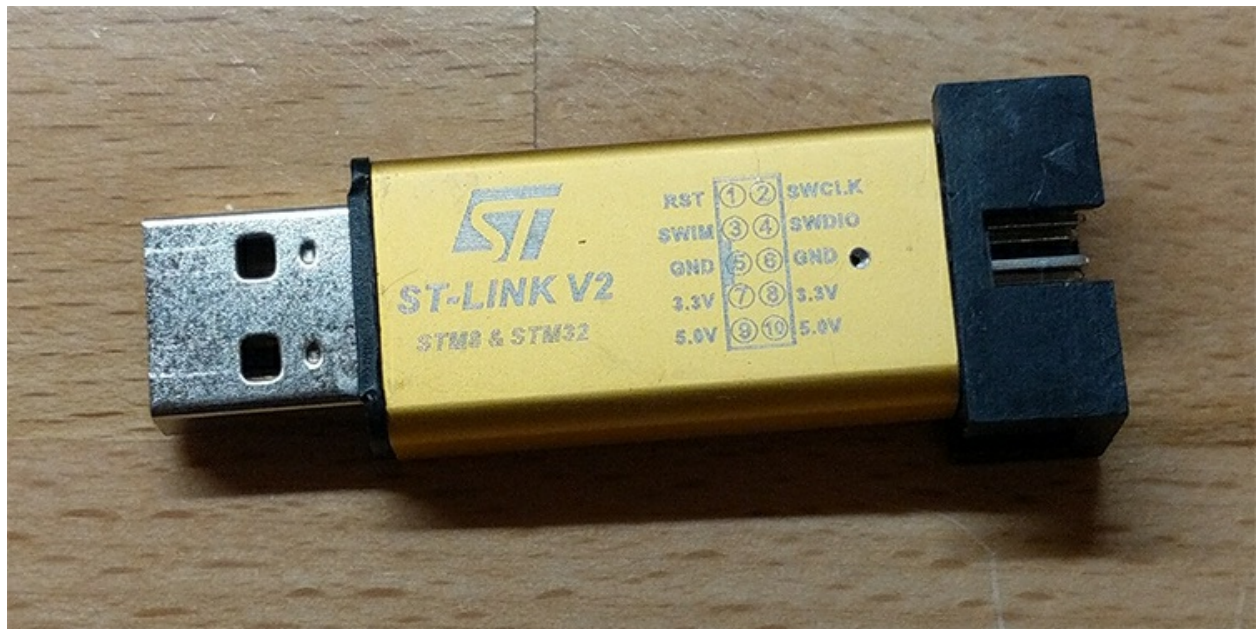
Figure 7-9: The mini ST-Link V2 programmer lets us interact with STM32 cores through SWD.
