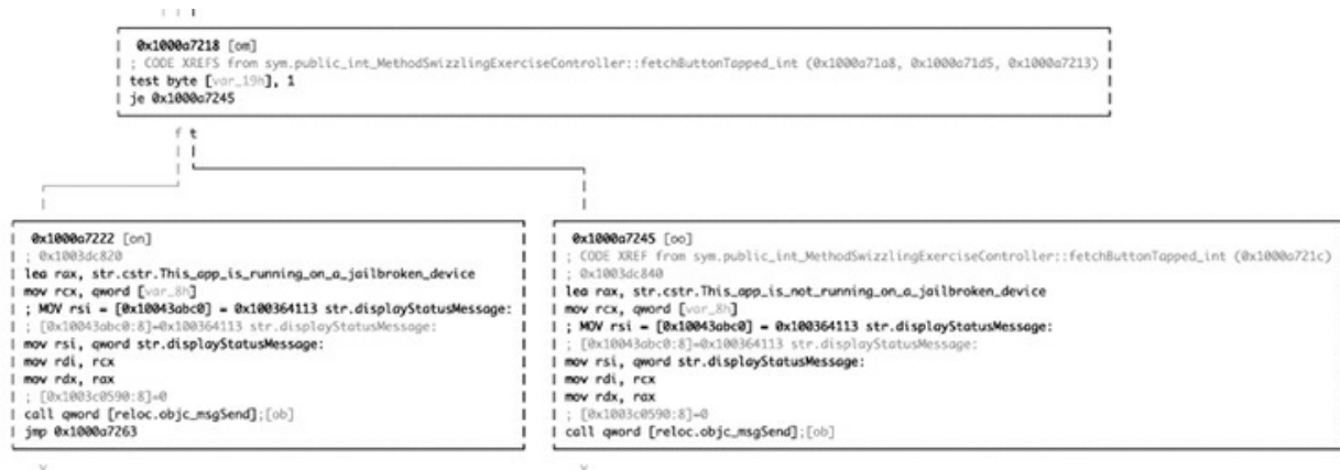
Figure 14-11: The Radare2 graph view representing the logic switch
