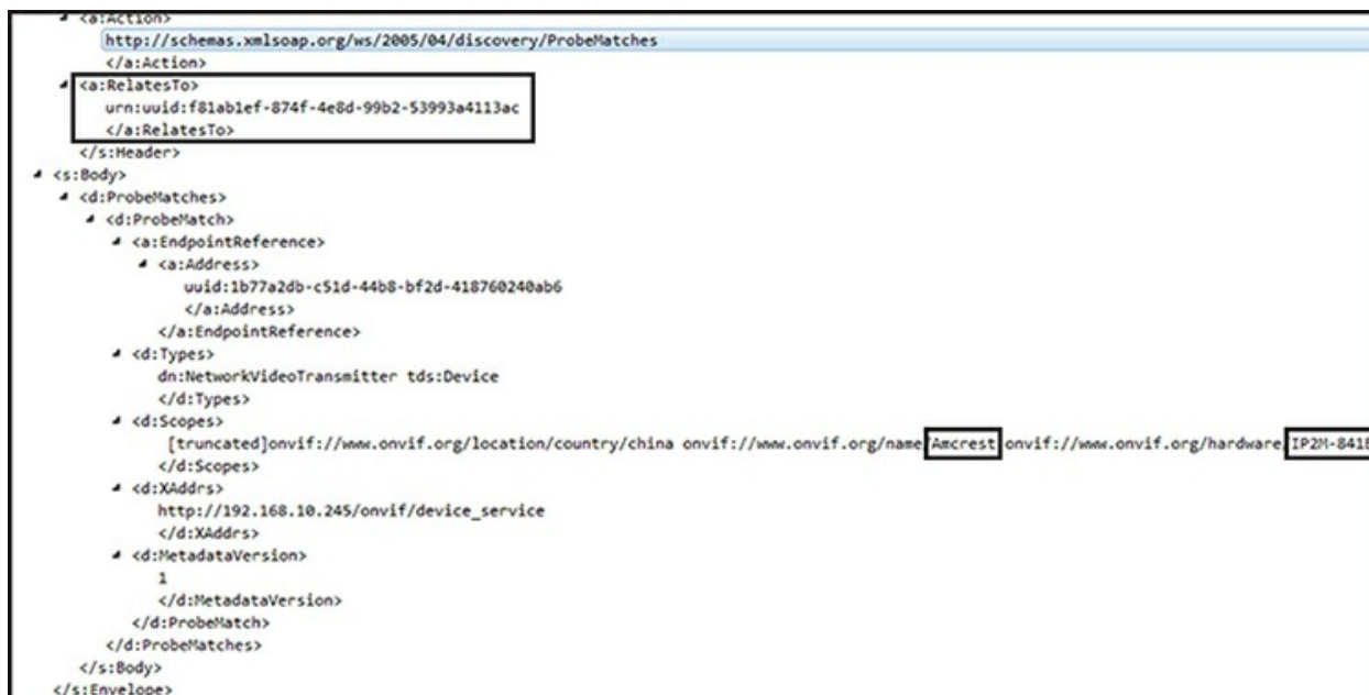
Figure 6-17: WS-Discovery Probe Match reply from an Amcrest IP camera on the network. Notice that the RelatesTo UUID is the same as the MessageID UUID that exacqVision sent.
